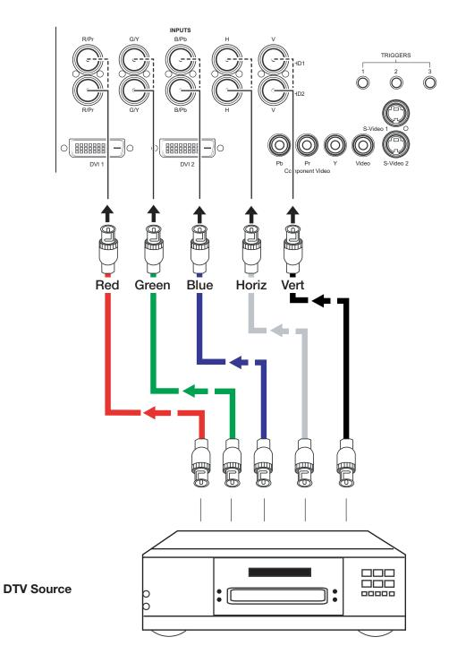
Figure 3-6. Digital (DTV) RGB Connections
